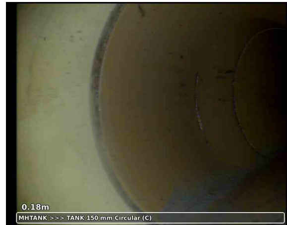
20240212-002705-snap0001.jpg, 00:00:24, 0.18 m Pipe size changes, new size(s), 100mm high
