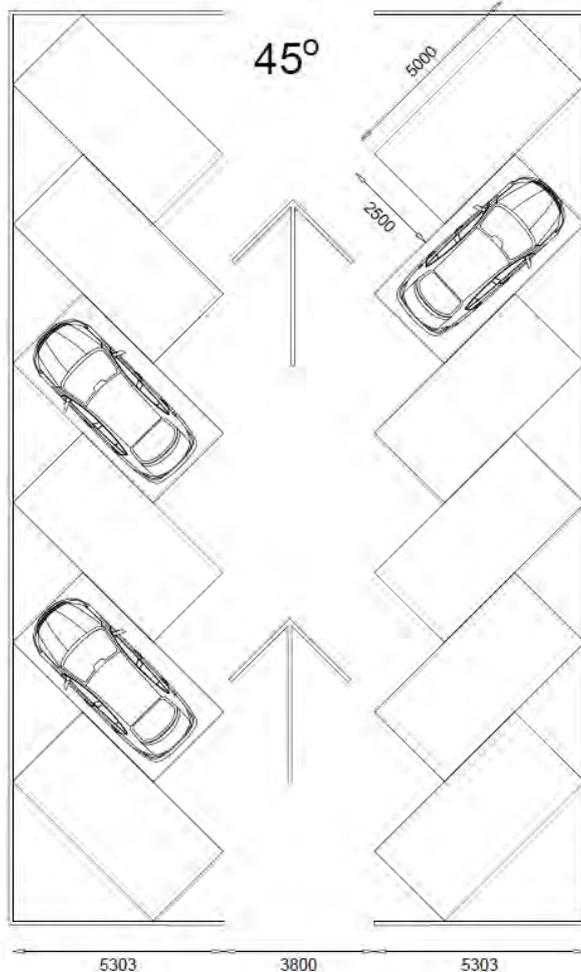
**Note: car spaces can only be interlocked properly at 45°**
